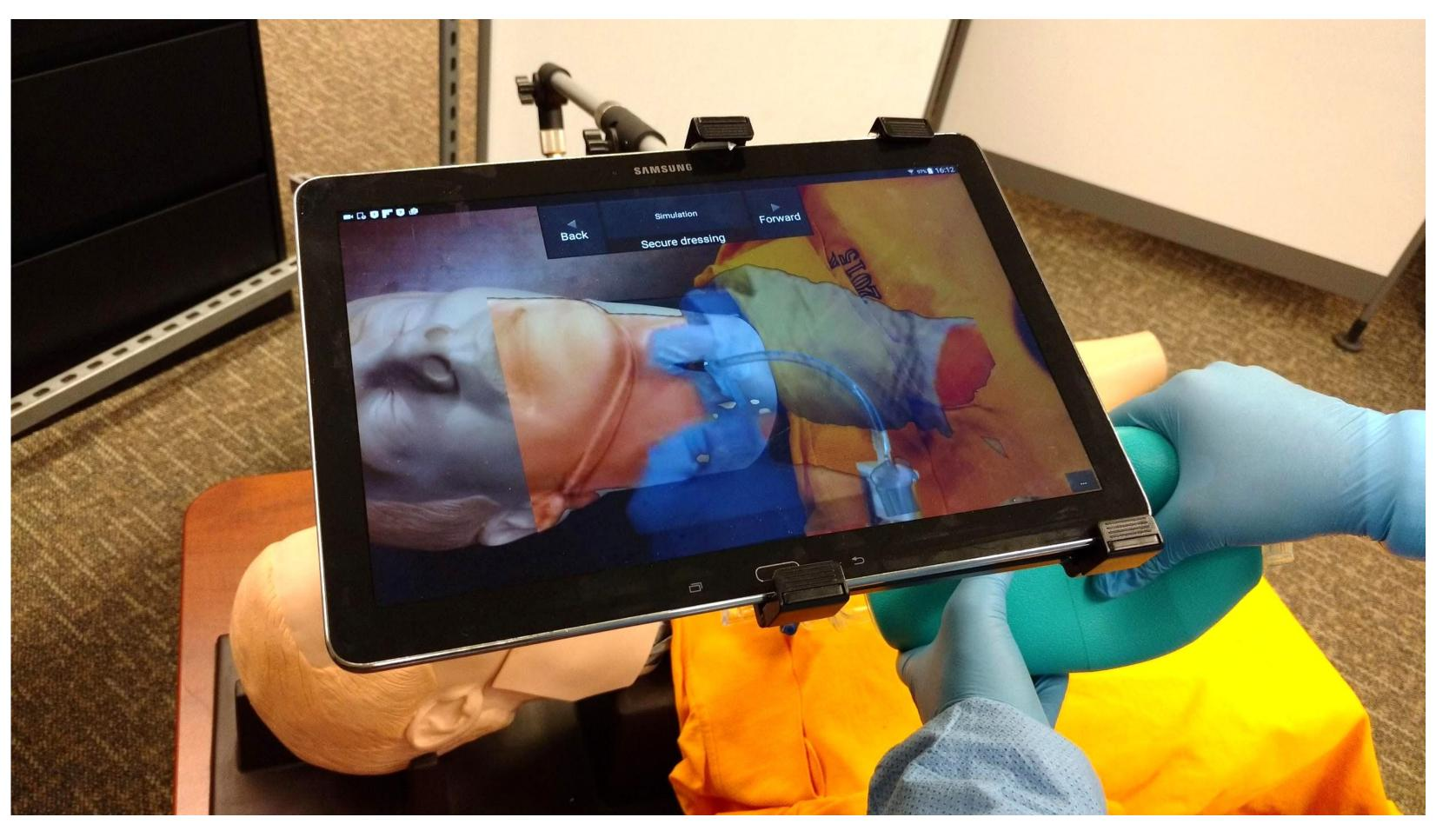
Figure 3. Trainee surgeon using an augmented reality transparent display (top), and trainee's view (bottom). The display overlays a visualization of a future step of a cricothyroidotomy procedure onto the simulator.
